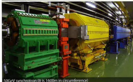
50GeV synchrotron (It is 1600m in circumference)
