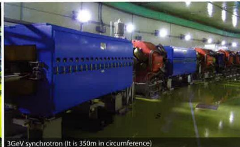
3GeV synchrotron (It is 350m in circumference)
